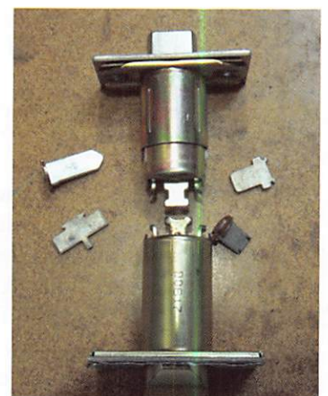
Photo 4: Two different spring latches. On the bottom is the passage version. On the top is the privacy latch with a different T-shaped retractor. Also included are 4 of the many tailpieces available from Marks USA
