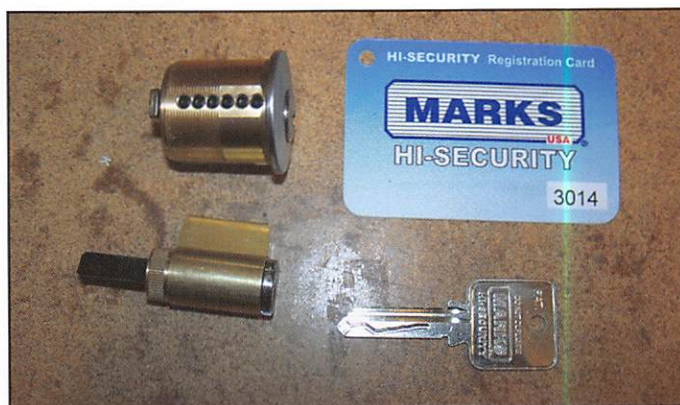
Photo 6 shows two of the new Hi-Security cylinders. The milling on the side of the key is for the finger pins that engage the sidebar.
